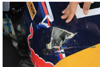
Crack on front body
